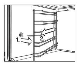
■ Pull the runners forwards out of the holder and remove, together with the catalytic side panels (if fitted).
